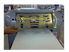
For unlocking the safety guard move the safety guard in the direction shown by the horizontal arrow and then move up or down the safety guard
