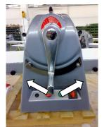
The roller gap is obtained by moving the handle on the right or on the left (*Fig. 6*). Each step of the handle on the toothed sector operates a different thickness. **THE ROLLERS CANNOT WORK IF THEY ARE IN CONTACT WITH EACH OTHER**.
