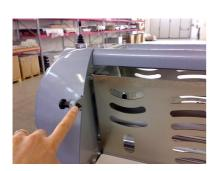
Pin for locking the tables when the tables are closed (Fig. 14)
