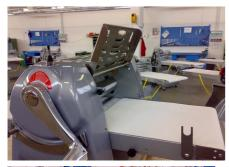
Safety guard open for replacing the scraper. In this case the machine can not working.
