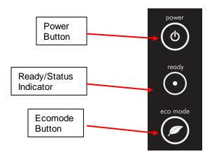
Figure 1: Machine User Interface
