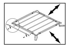
► Re-mount the side guide in accordance with the pass-through direction.
