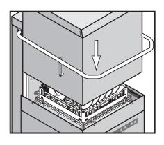
▶ Slide rack into the machine and close the hood.
