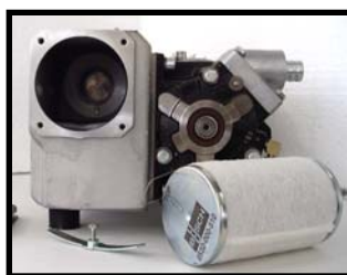
Remove tensioner and filter from the housing
