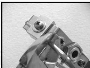
Pull the wire tight in second clamp plate using a pair of pliers and a vice.
